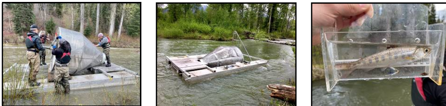
Figure 5: Photos showing: screw trap installation, operation and a sampled coho
