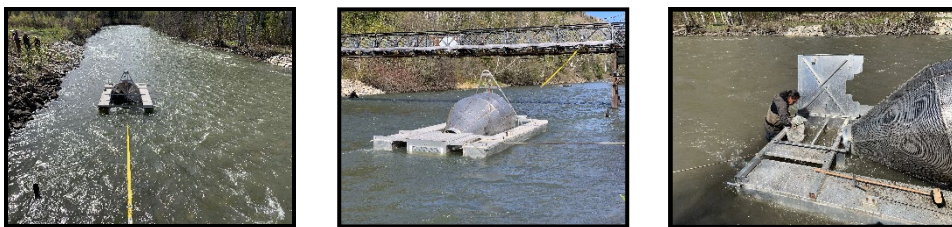
Figure 8: Photos showing rotary screw trap located downstream from the KSEF
