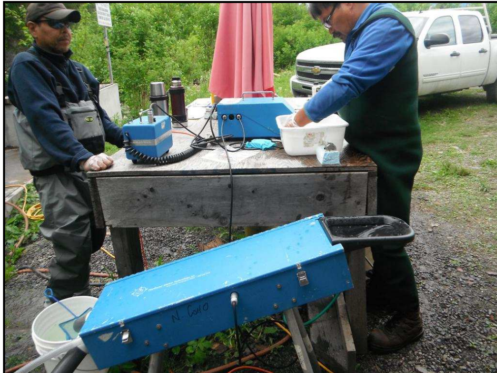
Figure 7: Photo of Coded Wire Tag (CWT) machine, Quality Control Device (QCD) and sampling station set-up.
