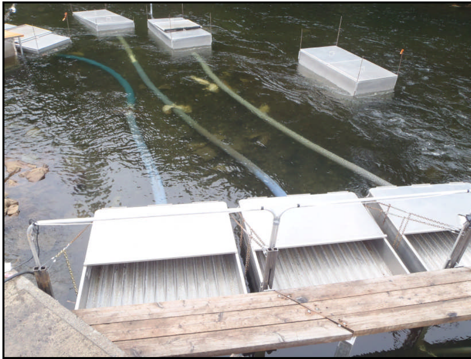
Figure 4: Photo of large holding boxes attached to smolt trap boxes with 6" hose.
