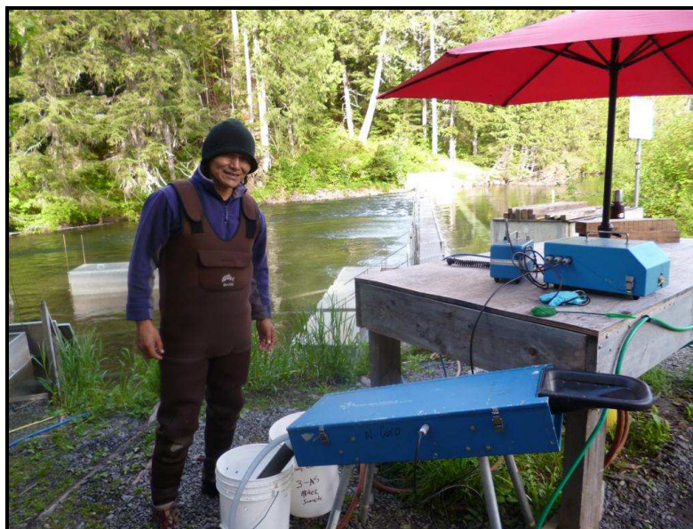
Figure 6: Photo of Coded Wire Tag (CWT) machine, Quality Control Device (QCD) and sampling station set-up.
