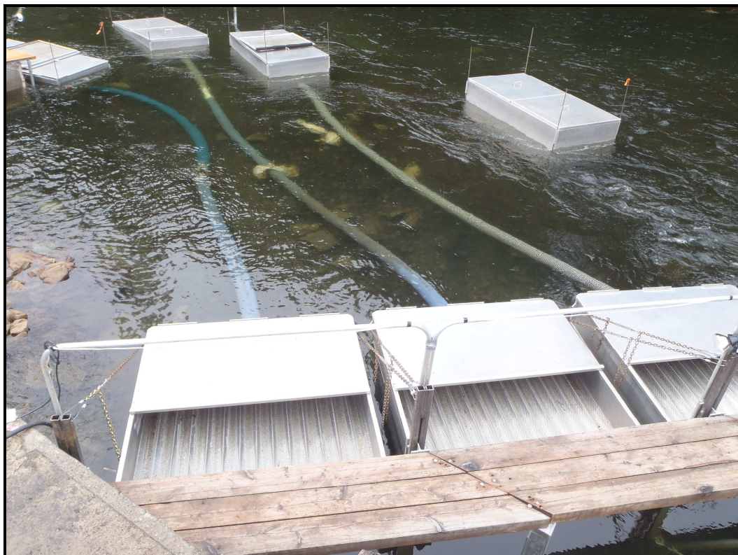
Figure 3: Photo of large holding boxes attached to smolt trap boxes with 6" hose.
