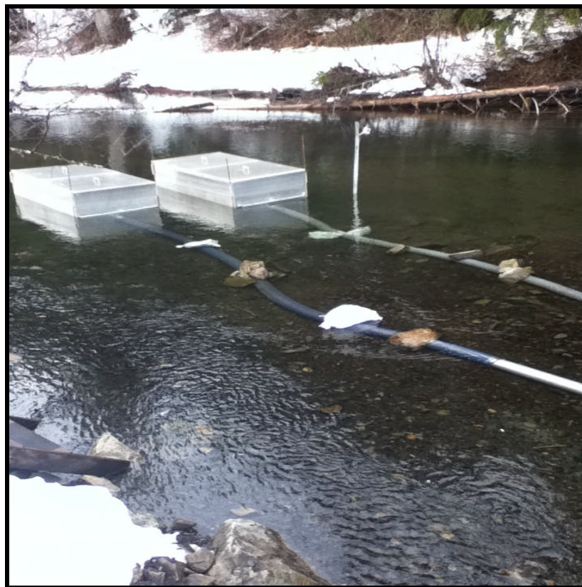
Photograph 2. Large holding boxes attached to smolt trap boxes with 6" hose.
