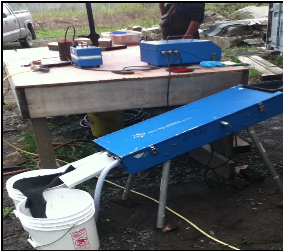
Photograph 6. Coded Wire Tag (CWT) machine, Quality Control Device (QCD) and sampling station set-up.
