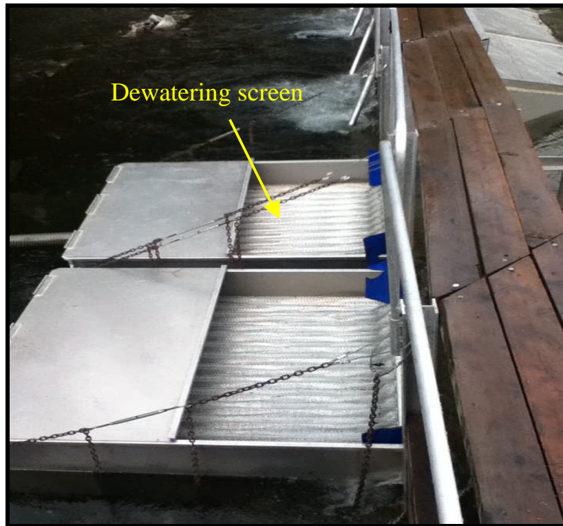
Photograph 1. Smolt trap box showing dewatering screen.
