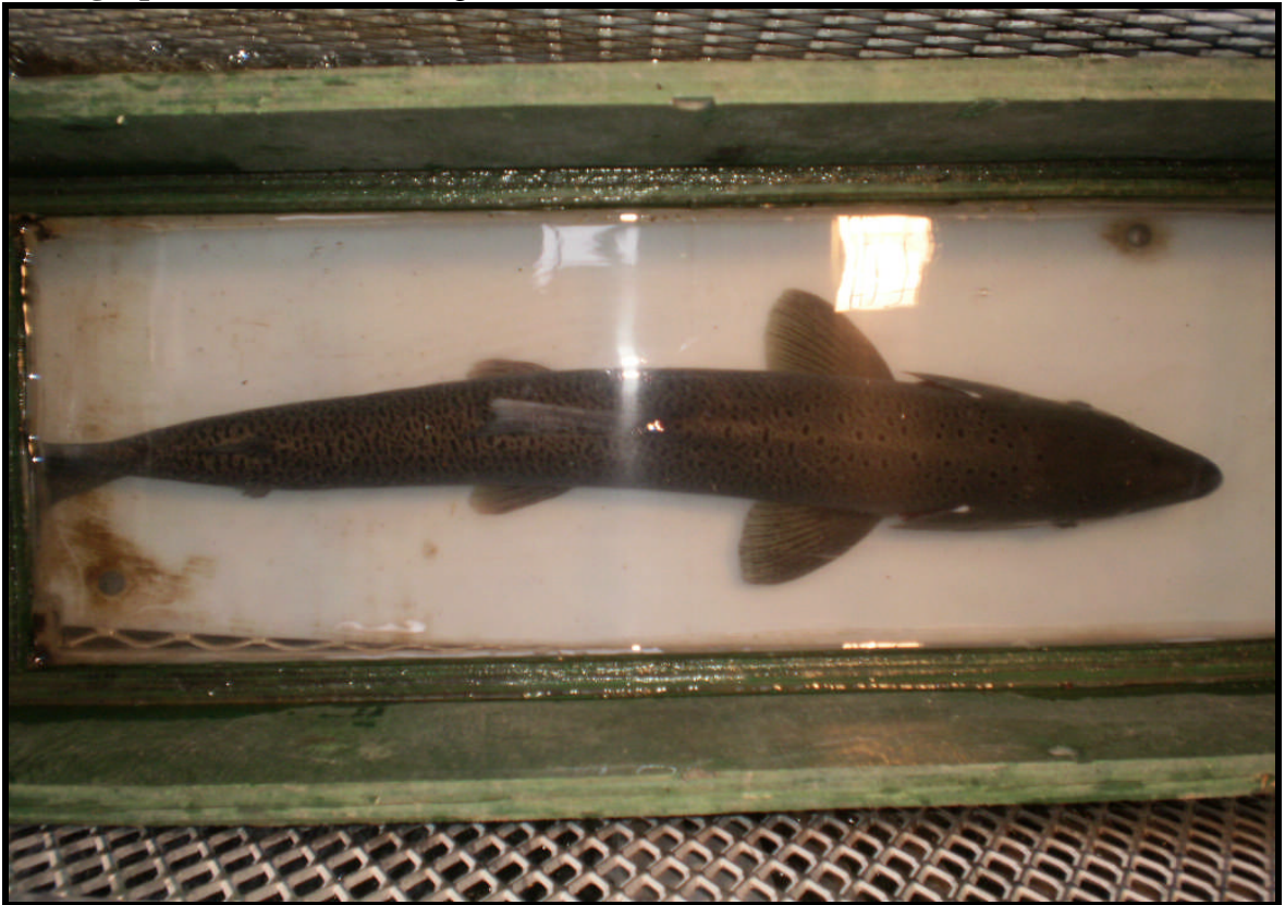
Photograph 6. Plexiglass viewing box used to identify fish species as it swims through the trap box.
