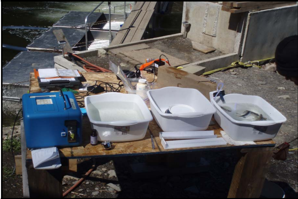
Photograph 6. Coded Wire Tag (CWT) machine and sampling station setup.
