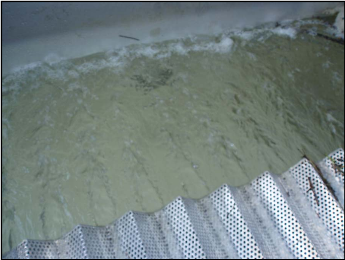
Photograph 1. Smolt trap box showing dewatering screen.
