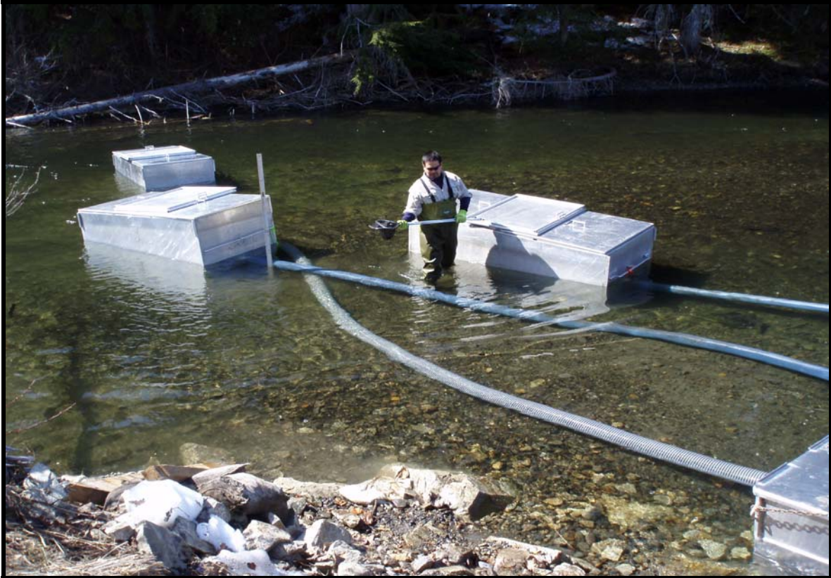
Photograph 2. Smolt traps connected to large holding boxes with 6" hose.
